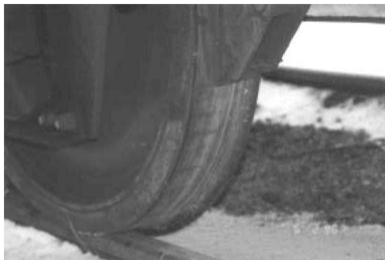
Fig. 4 Corrugation on the running surface of a cast iron block braked wheel
