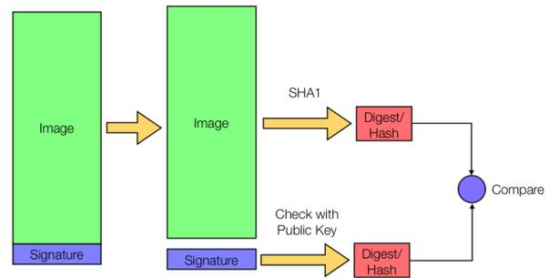
**Figure 3: Signature check: The image is hashed while the signature gets decrypted to return the original hash value. Both values then are compared.**
