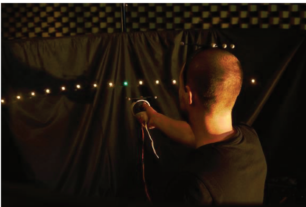
Figure 3: A test subject during the pilot studies. The listener extends their arm pointing to the location of the perceived sound object in the space relative to their self-body axes (egocentric pointing method).
