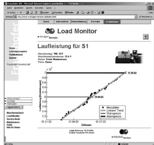
Fig. 4 Presentation of life cycle data (here: cumulated rotation speed) as a Web Service (copyright Fraunhofer IPK)
