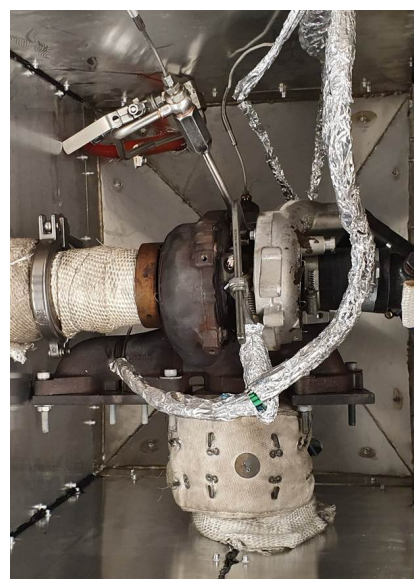
Figure 6. Setup of turbocharger inside the box, view from above.
