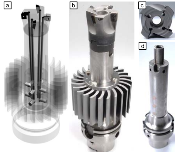
Fig. 1. Closed internally cooled milling tool (a) Model; (b) Tool; (c) Cutting head; (d) Cutter arbor with heat coupling elements
