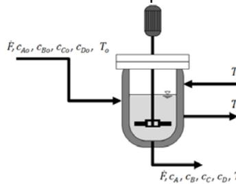
Figure 2. General scheme of the CSTR including all inputs and outputs.
