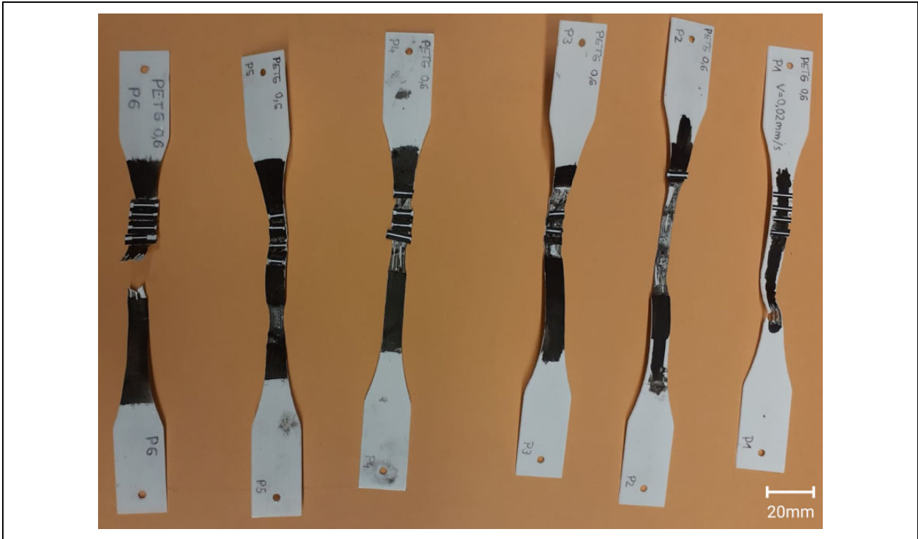
Figure 11. Inspection of the PETG specimens upon the uniaxial tensile tests.
